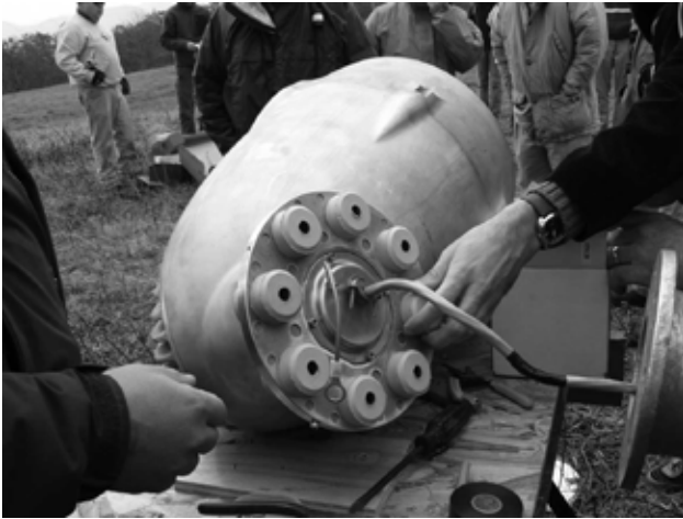
Fig. 11 Placing vibration isolators
